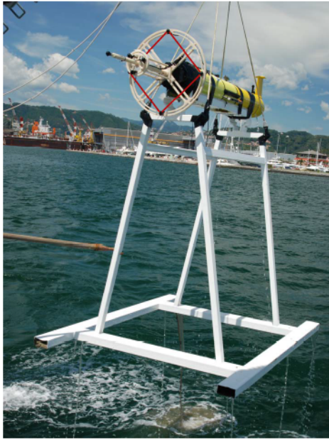
Figure 7. Slocum glider with acoustic antenna while it is recovered by using CV Leonardo after static measurements in La Spezia harbour. The glider is hosted by a metallic frame which can be deployed on the seabed. A red box outlines the diamond geometry of four of the eight hydrophones.
