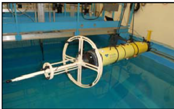
Figure 1. The CMRE Slocum glider equipped with the acoustic volumetric array plus a rear hydrophone (in front of the fin). Photo taken during preliminary water tank tests at CMRE.
